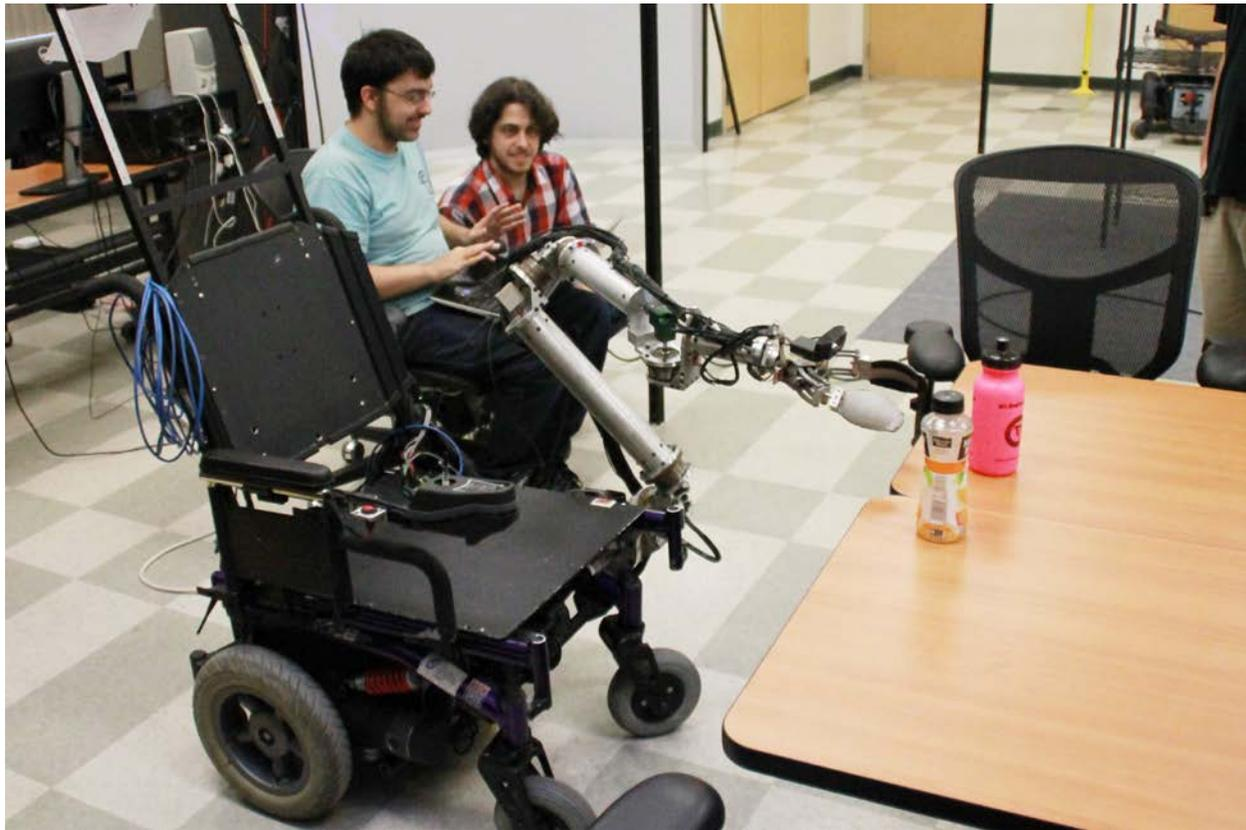
Wheelchair-Mounted Robotic Arm Controlled by a Brain-Computer Interface
